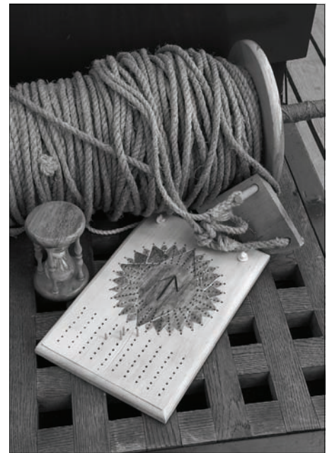
During long ocean voyages, the chip log was used every half hour to find the ship's speed. The speed was then recorded on a traverse board.
